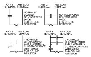
**NOTE:** This option should be selected if either Normally Closed (NC) or Normally Open (NO) detection devices or contacts are being used.
